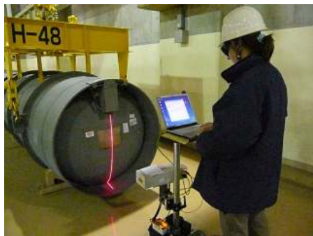
Figure 6: L2IS unit 1 scanning a 48Y cylinder: portable and operated by IAEA Staff.
